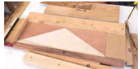
▲ Pic.11 For jointing, I used the biscuit jointer and the same jig to assemble and glue up the components for the carcass panels
